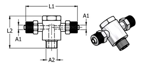
Hose diameter A1 = 6/4L1 = 33.0L2 = 17.5NV = 8Thread A2 = M5
